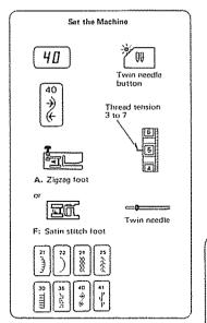
Your Kenmore 100 Stitch is equipped with a twin needle that can be used to sew parallel rows of straight or decorative stitches adding an exquisite touch to table linens and clothing.
